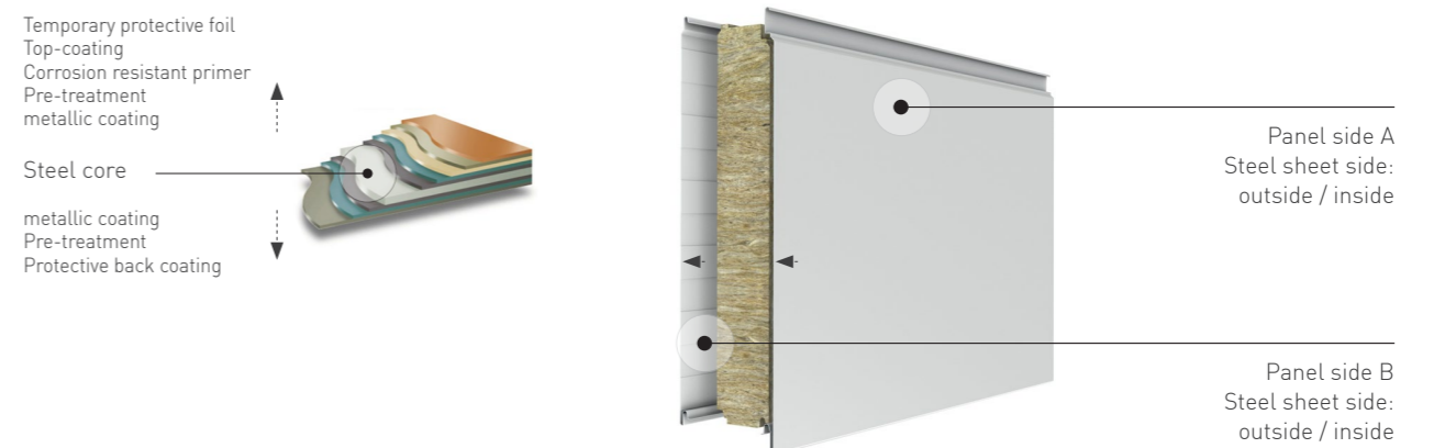
Fig. 2.1: Panel composition and coating structure example
